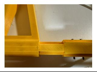
Step 5: Connect a long male connector (Bow Segment 3) to the end of the female connector (Bow Segment 1) and fit the nails in accordingly.
