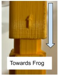
Step 4: Connect another female connector (Bow Segment 1) to the other end of Bow Segment 4 and fit the nails in accordingly.
