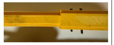
Step 3: Slide the Bow Truss down the short male connector until it hits the end. Make sure that the side labeled "F" is pointing towards the Frog connector.
