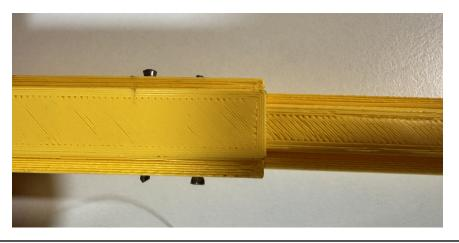
Step 6: Attach the Bow Tip to the end of Bow Segment 3 (the long male connector) and fit the nails in accordingly.
