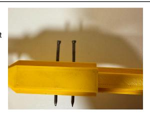
Step 2: Connect Bow Segment 1 (a female connector) to the end of Bow Segment 4 (the short male connector) and hammer in the nails by following the same procedure as in Step 1.
