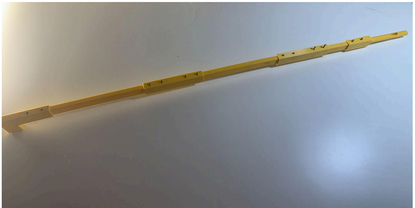
Fig 3: Prototype V3 printing in process. Larger, rectangular connectors using PLA plastic. Used nails for connectors instead of plastic components for greater durability.
